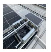
Large photovoltaic array cleaning robots Aluminum alloy bracket for stable Movement Without manual cleaning
